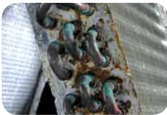
Copper tube and galvanized steel tube sheet after 500 hours in a controlled corrosive environment.
